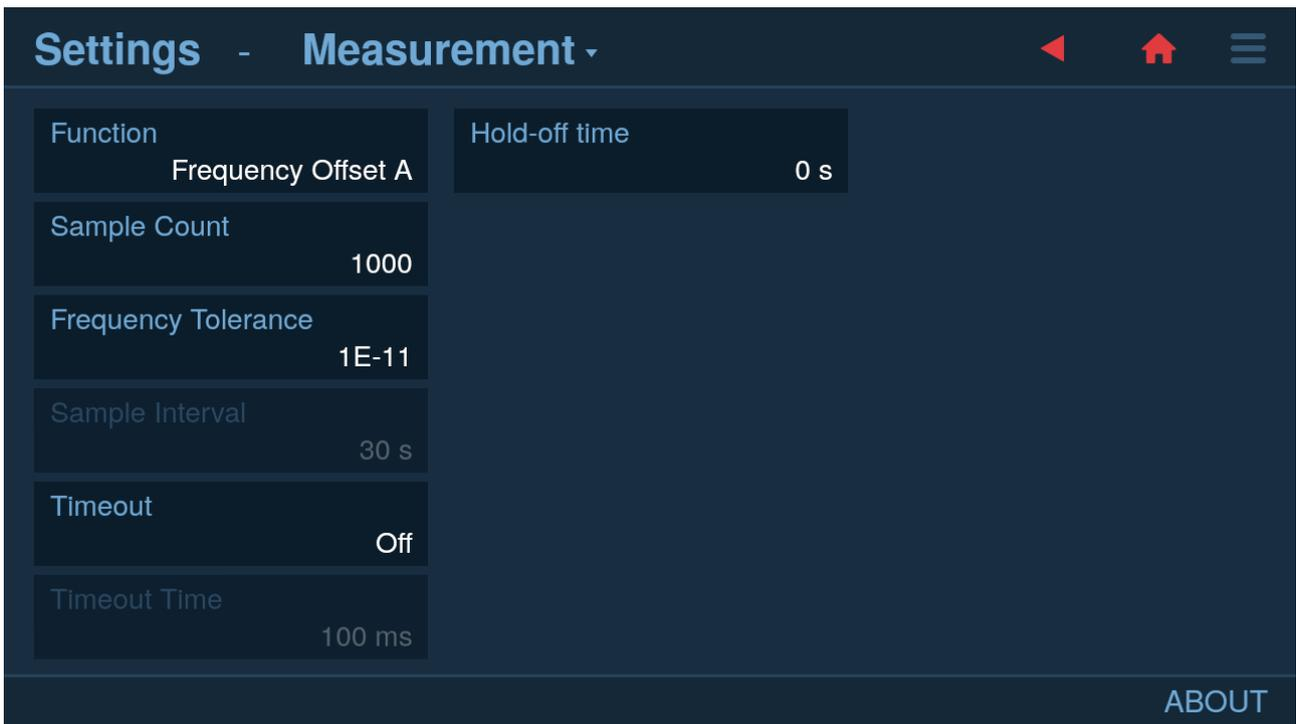
Fig. 4.4: Setting calibration tolerance for Frequency Offset function (Frequency Tolerance setting)
