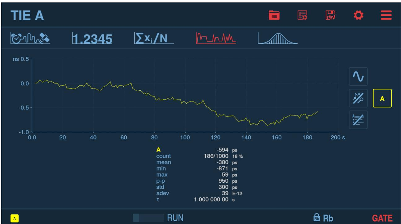
Fig. 4.6: Example of TIE measurement trend graph
